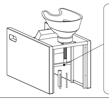
Connect the power plug. (Ombra with motorised legrest) Connect the pipes(drainage, water and hot water pipe) to the water mains.
